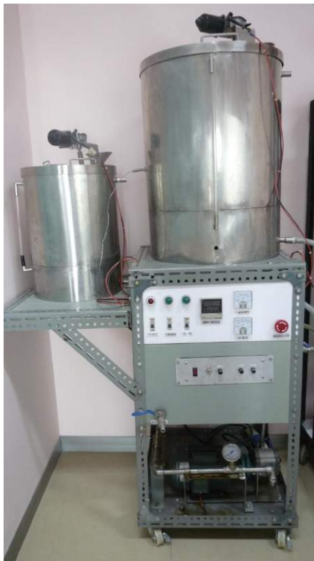
Fig. 4 Continuous ultrasonic biodiesel reactor designed by Untoro and Dimiyati, suitable for small scale and medium biodiesel plant.
