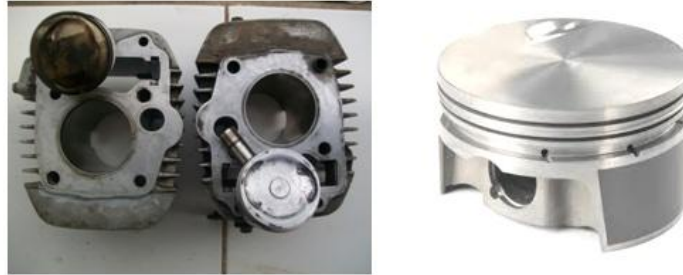
Figure 4. Cylinder and plunger (piston)
