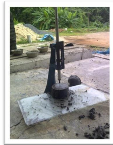
Figure-2. Vicat test equipment to determine the consistency and setting time
