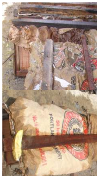
Fig. 7: Curing specimen beams
