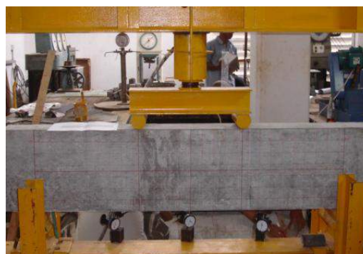
Fig. 8: Beam loading method
