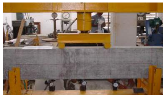
Fig. 8: Beam loading method
