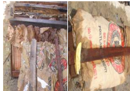
Fig. 7: Curing specimen beams
