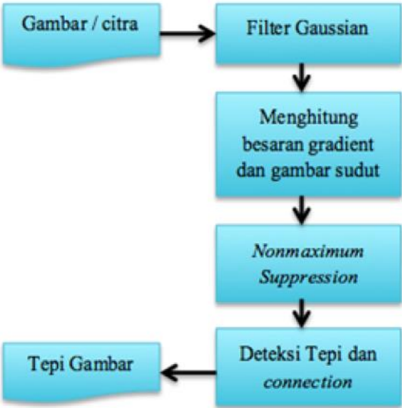
Figure 1. Steps Canny Edge Detection.
