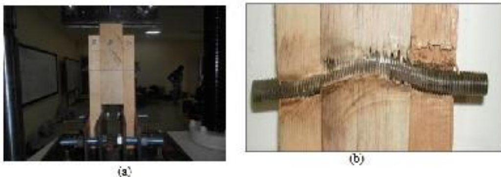
Figure 7. (a) Symmetric double shear connection tensile test photo (b) The bolt after the connection tensile test takes place of the IIIs yield mode.
