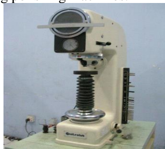
Figure 4. Tool Hardness Testing Vickers
