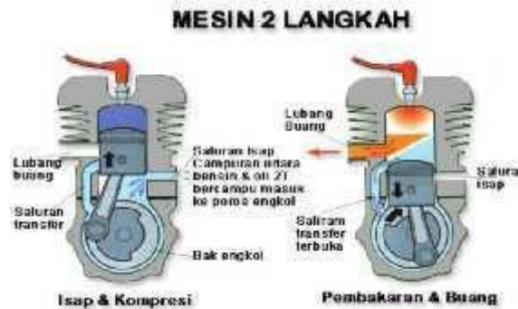
Figure 2. The working principle of the motor fuel picture petrol 2-step; (a) step suction and compression; (b) the power stroke and exhaust.
